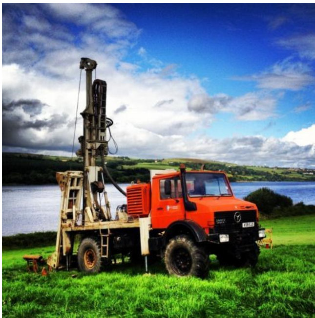
Photo: Coring rig on the banks of the Foyle River
