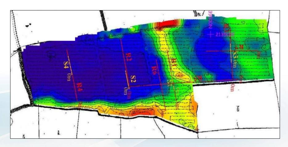
**EM31** Survey – Overburden Thickness, Karst, Structure etc.
