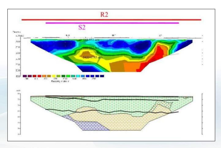
2D Resistivity and Seismics – Sand and Gravel
