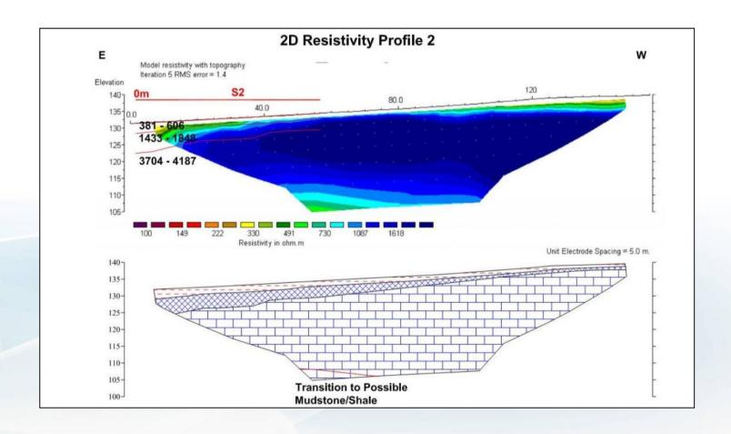
2D Resistivity and Seismics – OB and Bedrock
