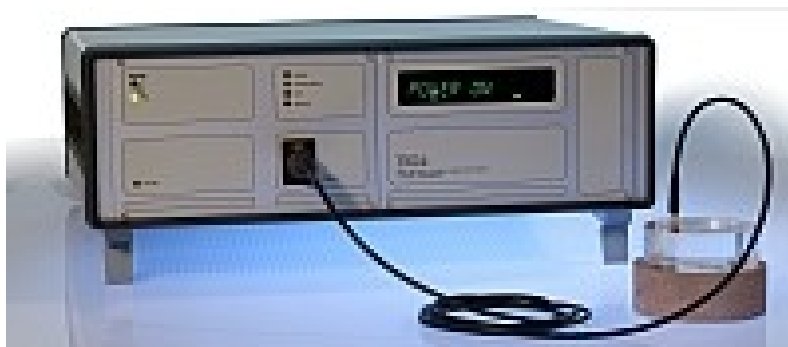
Figure 13: Thermal Conductivity Meter TK04 with HLQ probe used for measuring the heat conductivity of rocks.
