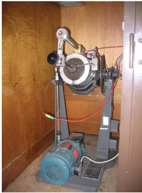
Figure 14: Dickson-type rocking autoclave used for high temperature experiments up to 200°C at BGS.
