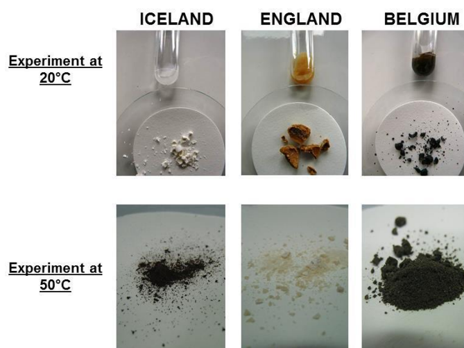
Figure 7: Precipitates formed during the GDEx treatment of three different simulated geothermal brines at two different temperatures.
