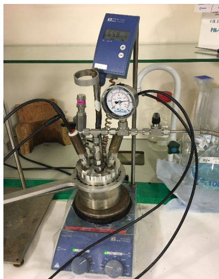
Figure 6: Elevated temperature and pressure stationary electrode reactor used for metal recovery studies.
